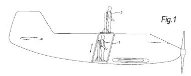
(57) Abstract: A safety support that comprises or is operably engagable with a safety harness for a person performing a stunt; wherein at least part of the support is movably mounted so that it can be moved from a first position where said person is located relatively safely for take off or landing, to a second, relatively exposed position, where said person can perform said stunt.
