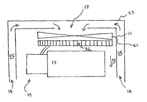
26 is a heat exchanger for a liquid cooled utility engine.
