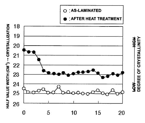
INTERFACE WITH METALLIC SHEET  $\leftarrow$  MEASUREMENT POSITION ( $\mu$  M)  $\rightarrow$  SURFACE
