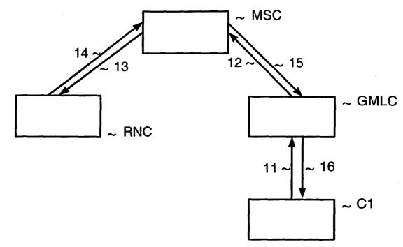
(57) Abstract: The invention relates to the provision of deferred location reporting wherein the reporting is triggered by a trigger location change event. Trigger location change events are either related to a user of a cellular telecommunication network entering, leaving or changing an area, or to an area, which is entered or left by a user.
