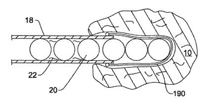
(57) Abstract: A system for forming an implant to stabilize an interior of a vertebral body is provided. The system includes a delivery cannula (18) in which there is an agglomeration of beads (20) and cement (22). A membrane is disposed over the open end of the cannula. When the agglomeration is discharged from the cannula it fills the membrane. The membrane thus forms the outer shell of the implant internal to the bone.
