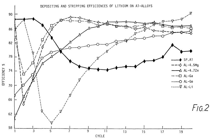
lmA/cm2 1 Coulomb Propylene Carbonate/LiBF4 500 second delay between charge/stripping
