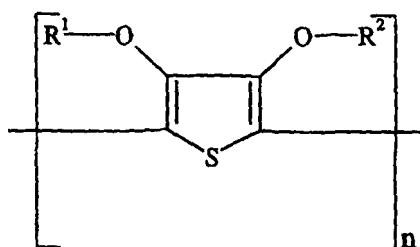
in which, each of R<sup>1</sup> and R<sup>2</sup> independently represents hydrogen or a C1-4 alkyl group or together represent an optionally substituted C1-4 alkylene group or a cycloalkylene group.
