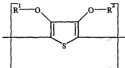
in which R<sup>1</sup> and R<sup>2</sup> independently of one another represent hydrogen or a C1-C4 alkyl group or together form an optionally substituted C1-C4-alkylene residue, in the presence of polyanions.
