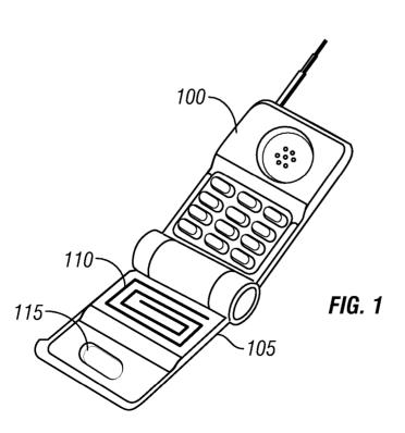
(57) Abstract: A deployable antenna used in a mobile device. The antenna can be folded into a stowed position in which it is coplanar with the housing. It can also be unfolded, preferably to an oblique angle, and used to receive wireless power from at least 6 inches away.
