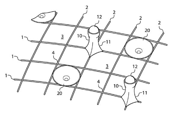
(57) Abstract: A massaging garment worn in close proximity to a wearer's skin is made from a Sretchable fabric havign a plurality of fibers (1, 2). Pushing elements (12) for pushing the wearer's skin away from the stretchable fabric and pulling elements (20) for pulling the wearer's skin toward the stretchable fabric are secure thereto. The pushing and pulling elements (12, 20) produce a massaging effect on the wearer's skin.
