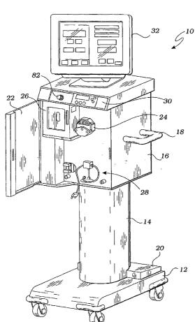
**(57) Abstract:** A system utilizes an oxygenation device to generate a gas-enriched physiologic fluid and to combine it with a bodily fluid to create a gas-enriched bodily fluid. The oxygenation device may take the form of a disposable cartridge, which is placed within an enclosure. An electronic controller manages various aspects of the system, such as the production of gas-enriched fluids, flow rates, bubble detection, and automatic operation and shut down.
