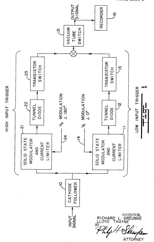
VOLTAGE LEVEL MONITORING DEVICE
