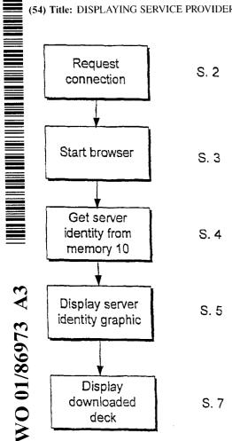
(57) Abstract: A mobile cellular telephone handset (1) is WAP enabled. Browser connection settings are configured so that whilst connection is being made to a WAP server, the user is provided with a graphical display that indicates the identity of the service provider for the server.
