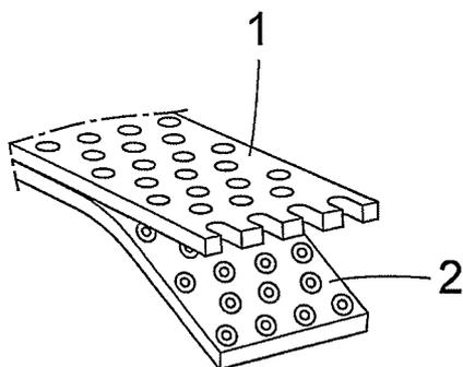
(57) Abstract: The present invention relates to a method for making holes in a layer (1) of heat-fusible material. According to the invention a layer of absorbent material (2) is placed in contact with a layer (1) of heat-fusible material, following which the layer of heat-fusible material is heated locally so that holes are formed in the material.
