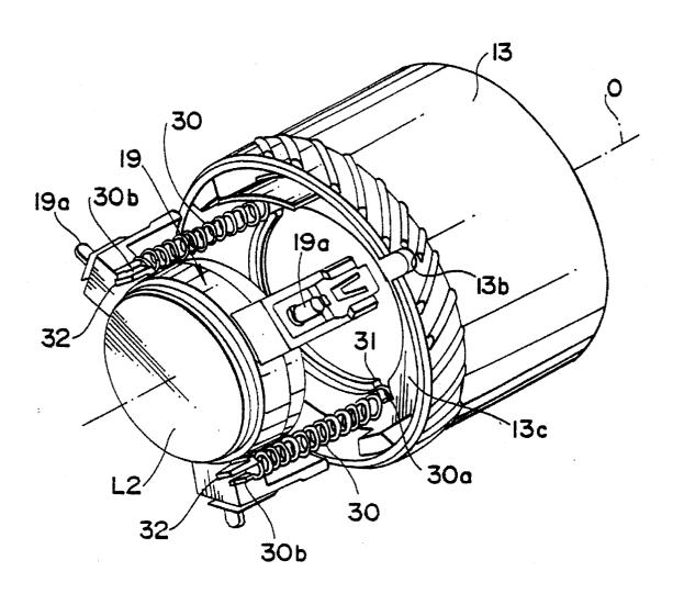
BACKLASH REMOVING MECHANISM FOR ZOOM LENS ASSEMBLY
