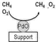
tem is configured such that a ceramic substrate is impregnated with palladium-impregnated first alumina, platinum-impregnated second alumina, and a ceria component, wherein the first alumina is further impregnated with a cocatalyst selected from the group consisting of barium, nickel, lanthanum, samarium, and yttrium, thus significantly inhibiting the deactivation of the CNG lean burn engine catalyst.
