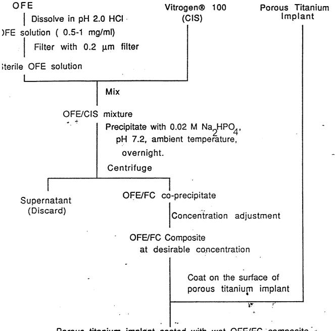
Porous titanium implant coated with wet OFE/FC composite
