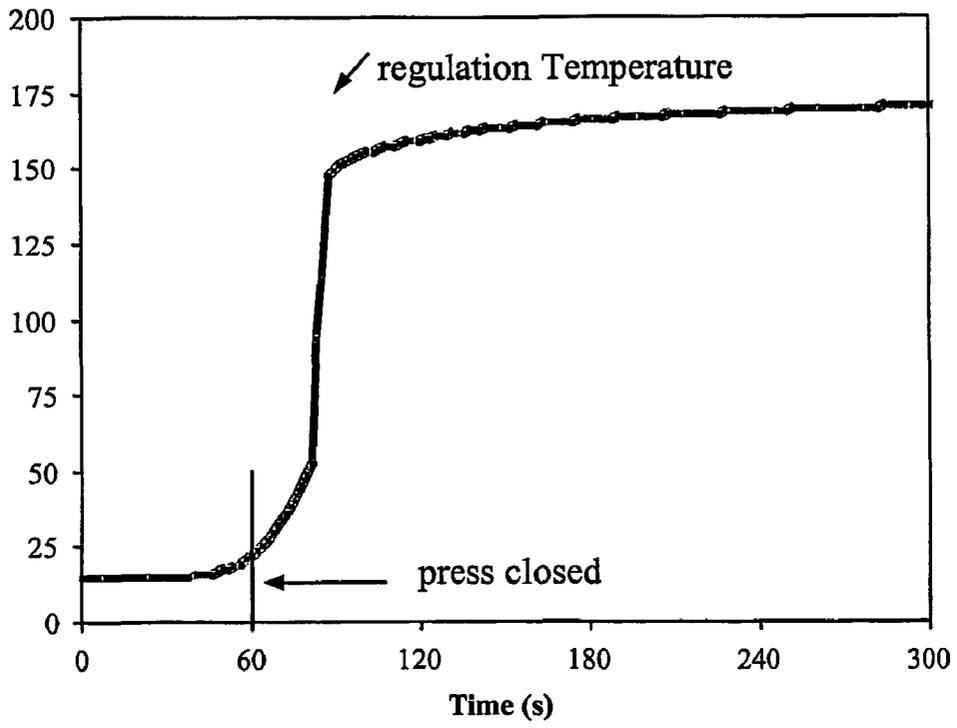
[0080] FIG. 1: Core temperature evolution during pressing of gluten and wood particles. 175° C. regulation temperature, 300 g wood (9% MC), 60 g gluten (7% MC)
