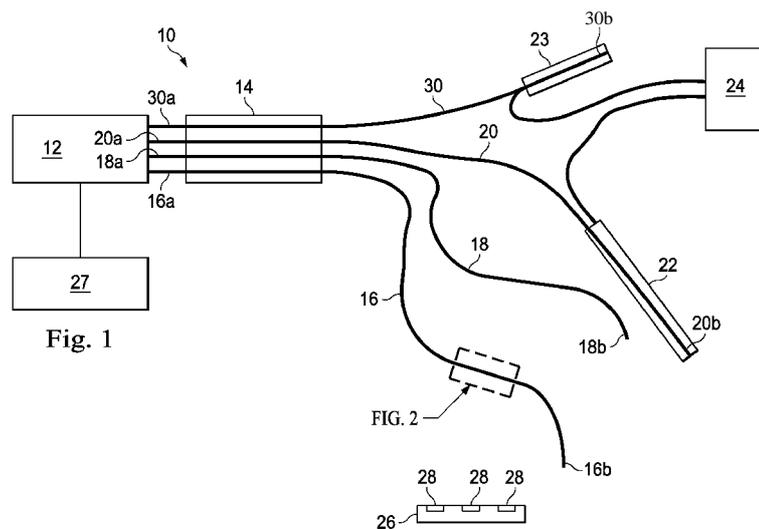
(57) **Abstract:** A method comprises receiving first shape data from a first elongated optical fiber section in a first shape sensor. The first elongated optical fiber section extends between a reference fixture and a first anatomic fixture coupled to a patient anatomy. The method further comprises determining a pose of the first anatomic fixture from the first shape data and tracking a pose change for the first anatomic fixture.
