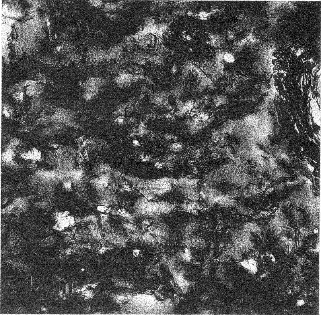
5 wt% 1000 m 2 /g expanded graphite in EVA copolymer
