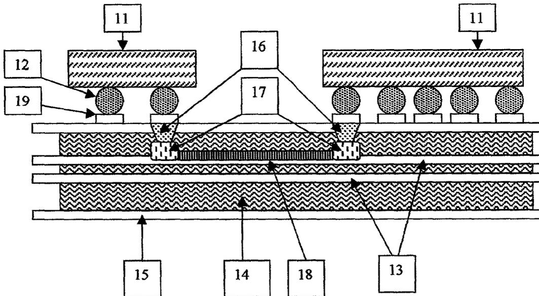
**Printed Circuit Board Containing Optical Elements**
