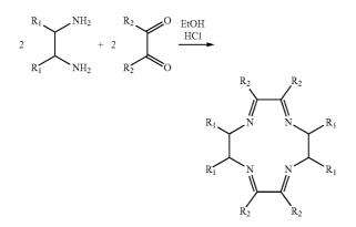
In Scheme II, where the diamine is 1,2-di-amine-benzene and the R2 group of the diketone is a phenyl group, the N4 macrocycle is DTTCT, which can form a copper complex as shown below:
