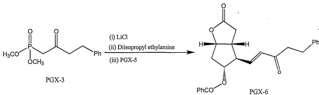
The phosphonate ester ( PGX-3) (176.2g, 0.69M, 0.95eq.) was dissolved in dry acetonitrile (1.8L) in an inert atmosphere and lithium chloride (153.4g, 3.62M, 5.0eq.) added. The mixture was cooled to approximately -15°C and dry diisopropyl ethylamine (178.1g, 1.38M, 1.9eq.) added over 10 minutes
