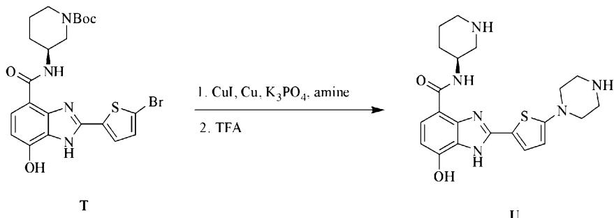
Compound T was reacted with the requisite amine in the presence of copper and copper (I) iodide followed by deprotection to afford compound U (Scheme II).
