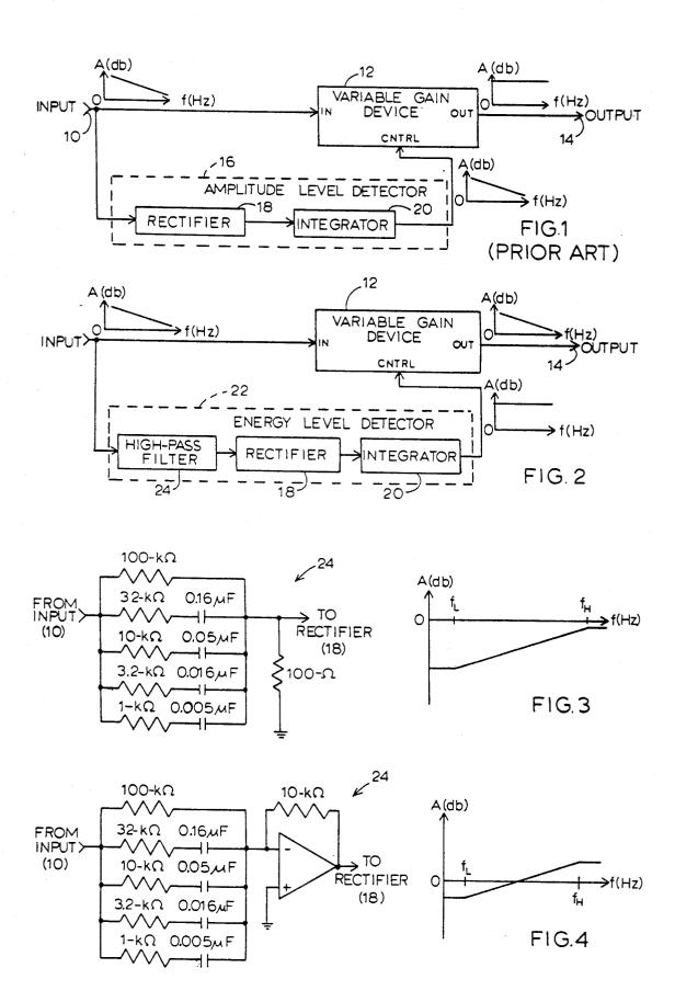
**AUDIO SIGNAL ENERGY LEVEL DETECTION** METHOD AND APPARATUS
