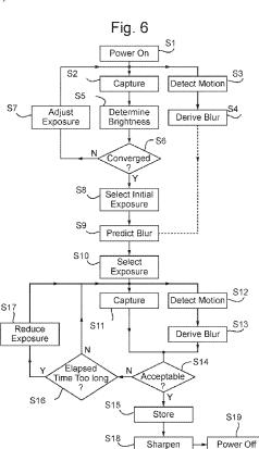
(57) Abstract: A camera unit that comprises an image sensor and a motion sensor performs an image capture operation in which still images are captured intermittently without triggering by a user. It is determined whether a captured image is of acceptable quality taking into account at least the degree of blurring indicated by the detected motion. If so, the captured image is stored, or else further images are captured until an image of acceptable quality is captured and stored.
