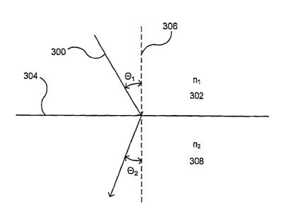
(57) Abstract: An optical device includes an interface (304) between two or more media (302 and 308). The refractive indices (n1 and n2), orientations of media, and alignment relative to a propagating wave (300) define a refractive boundary at which reflections may be reduced or eliminated, and at which, for certain incident angles, rays may be refracted on the same side of the normal (306) as the incident ray (300).
