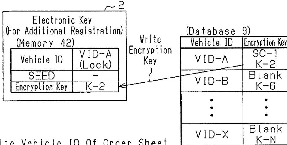
Write Vehicle ID Of Order Sheet And Encryption Key Corresponding To Vehicle ID From Database
