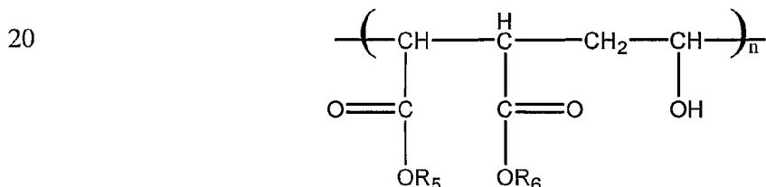
25 wherein R<sub>5</sub> and R<sub>6</sub> are individually and respectively selected from the group consisting of H, the alkali metals, NH<sub>4</sub> and C<sub>1</sub>-C<sub>4</sub> alkyl ammonium groups (and most preferably, H, Na, K and NH<sub>4</sub> depending upon the application), and n ranges from about 1-10000 and more preferably from about 1-5000.
