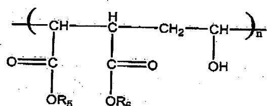
wherein R<sub>5</sub> and R<sub>6</sub> are individually and respectively selected from the group consisting of H, the alkali metals, NH<sub>4</sub> and C<sub>1</sub>-C<sub>4</sub> alkyl ammonium groups, and n ranges from about 1-10,000.
