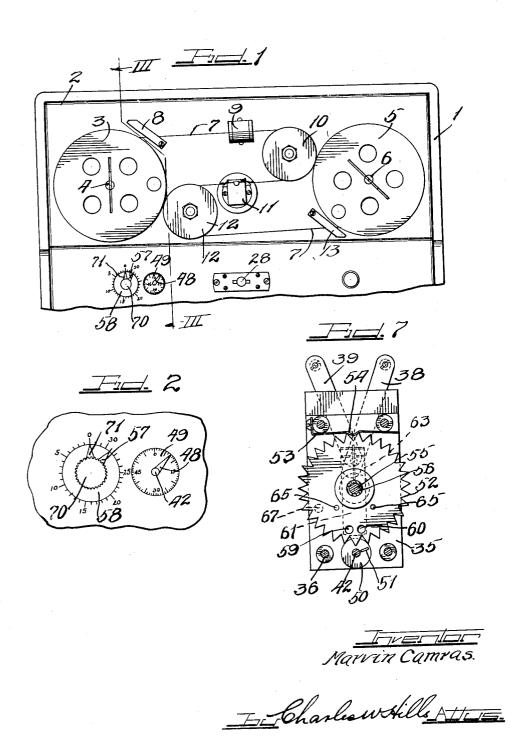
SAFETY TIMING MECHANISM FOR MAGNETIC RECORDERS
