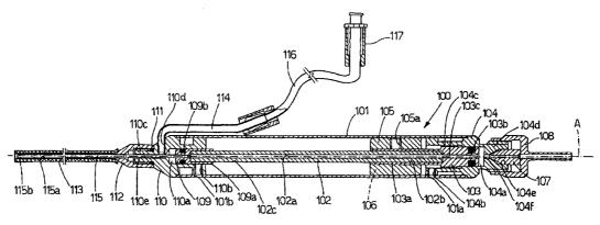
(57) Abstract: A lacrimal duct endoscopy unit (10) having a handset (100, 200) in turn having a device for optically detecting occlusions in the duct, and a device for surgically removing the occlusions. A lacrimal duct intubation device comprising a tubular portion having a conical flared portion at its proximal end and a tapered distal end.
