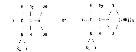
where R<sub>1</sub>, R<sub>2</sub>, and R<sub>3</sub> are independently hydrogen or C<sub>1</sub>-C<sub>4</sub> alkyl; n is 2-4; X is aryl, substituted aryl or C<sub>1</sub>-C<sub>6</sub> alkyl; Y is selected from the group consisting of hydrogen, amine protecting group, and amino acid, dipeptide or tripeptide linked through the C-terminal carboxylic acid.
