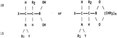
where R<sub>1</sub>, R<sub>2</sub>, and R<sub>3</sub> are independently hydrogen or C<sub>1</sub>-C<sub>4</sub> alkyl; n. is 2-4; X is aryl, substituted aryl or C<sub>1</sub>-C<sub>6</sub> alkyl; Y is selected from the group consisting of hydrogen, amino acid, dipeptide or tripeptide
