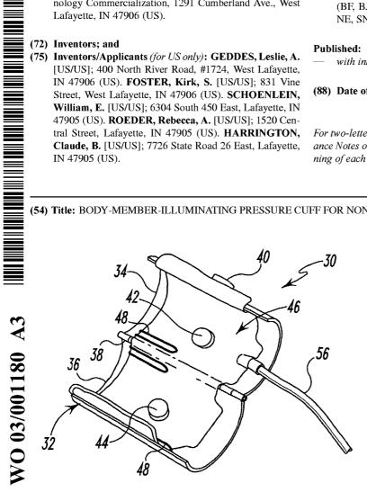
(57) Abstract: A member-illuminating cuff (30) for measurement of systolic, means and diastolic pressure, oxygen saturation, pulse and respiratory rate in small body members, comprising a hinged cuff housing (32), one or more light sources (40, 42) mounted on a first section of the housing, a photodetector (44) mounted on a second section of the housing, and a disposable, inflatable cuff (46) adapted to fit within the cuff housing and around a body member placed therein.
