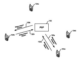
tional parameter and at least one timing parameter for the one or more measurements. In response to the request, the first device receives a measure report that includes measured values for each of the one or more measurements.
