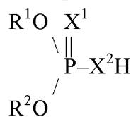
wherein the average total number of carbon atoms in hydrocarbyl groups  $R^1$  and  $R^2$  for the one or more phosphorus-containing compounds is at least 10.4. Although such approaches have provided a measure of success, the problem remains to provide adequate engine lubrication and at the same time further reduce phosphorus contribution to the exhaust and the corresponding risk for catalyst contamination. The present invention provides a solution to this problem.
