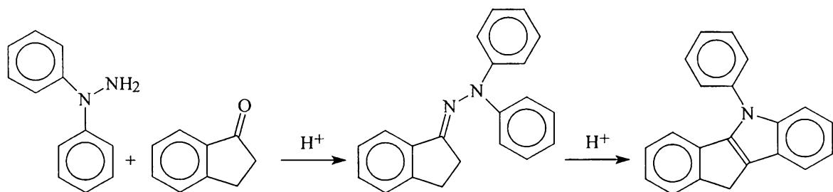
In a 0.25 l bulb were placed 13 g (70 mmol) of N,N-diphenylhydrazine, 9.2 g (70 mmol) of 1-indanone and the solution obtained by mixing 5 ml 96% H<sub>2</sub>SO<sub>4</sub> in 80 ml ethanol. The thus obtained mixture was heated at reflux for 4 hours and it was then poured into a solution of 7.5 g NaOH in 200 ml water.
