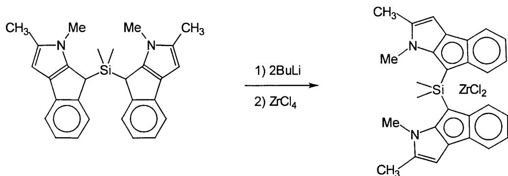
A suspension of 0.9g (2.1mmol) of the ligand prepared in Example 23 in 20ml of ether was treated with 2.7ml 1.6N BuLi in hexane, at room temperature. The resulting mixture was stirred for 3 hours and then treated with 0.49g (2.1mmol) of  $\text{ZrCl}_4$ . The red precipitate that formed was filtered and recrystallized from dichloromethane, thus giving 0.3g of the target compound (yield=25%).
