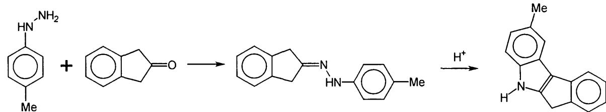
12.2g (0.1mol) of p-Me-phenylhydrazine, 13g (0.1mol) of indan-2-one and 100ml of isopropanole were placed into a bulb. The obtained mixture was refluxed for 1 hour; the mixture was then treated dropwise with a solution of 5ml  $H_2SO_4$  in 30ml of isopropanol and refluxed for 1 hour. The resulting mixture was cooled to room temperature and poured into water. The precipitate was filtered, washed with water and finally dried, thus
