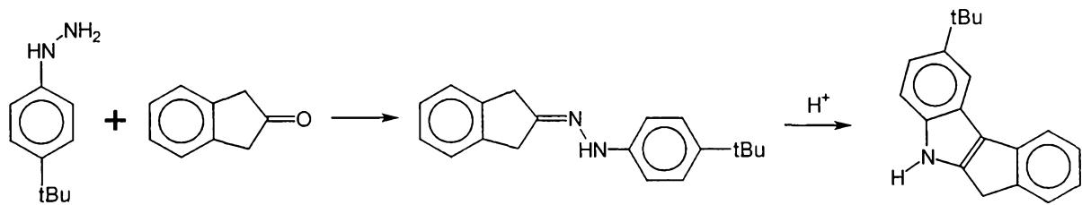
16g (0.1 mol) of t-butyl-phenylhydrazine, 13g (0.1 mol) of indan-2-one and 100 ml of isopropanole were placed into a bulb. The obtained mixture was refluxed for 1 hour; then it was treated dropwise with a solution of 5ml  $H_2SO_4$  in 30 ml of isopropanole and refluxed for 1 hour. The resulting mixture was cooled to room temperature and poured into water. The precipitate was filtered, washed with water and finally dried, thus yield 18g of 2-t-butyl-5,6-dihydroindeno[2,1-b]indole (yield = 69%).
