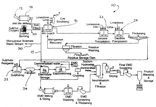
(57) Abstract: A process for the hydrometallurgical processing of manganese containing materials, the process characterised by the combination of a manganese dioxide containing feedstock and an acidic solution to form a leach solution, and passing a volume of sulphur dioxide gas through that leach solution, whereby the levels of dithionate ion generated in the leach solution are less than about 5g/l. Also described is a process for the production of electrolytic manganese dioxide.
