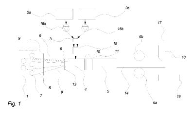
(57) Abstract: The invention relates to a process for manufacturing frames orsashes for windows or doors, the windows and doors comprising pultruded fibrereinforced polyurethane elements which are powder coated with UV-curing polyester powder.
