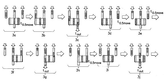
AVERAGE CYCLE TIME (AVERAGED OVER 3 SLABS)  $(t_{0.5 move} + t_{out} + 2 \times t_{0.5 move} + t_{out} + t_{0.5 move} + t_{out})/3 = 4/3 \ t_{0.5 move} + t_{out}$
