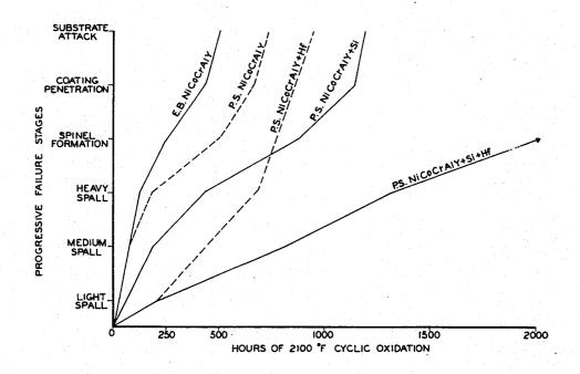
PROGRESSIVE FAILURE STAGES
