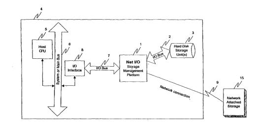
(57) Abstract: An apparatus and method implemented in embedded software that transparently redirects local hard drive requests to a Network Attached Storage (NAS) subsystem (15) is provided. The apparatus, contains a large front end cache used to intercept local hard disk (3) I/O requests at the lowest level before forwarding to an external attached NAS subsystem (15), providing a transparent high performance centrally managed storage solution.
