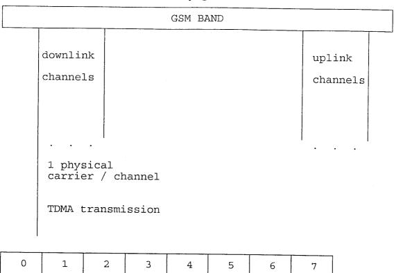
1 TDMA frame = 8 time slots, i.e. 8 logic channels
