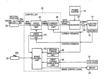
operation lever has been operated, on the basis of a differential between the second torque value and the first torque value, and which causes the brake to release the braking action on the winch drum by transmitting, to the brake, a control signal instructing release of the braking action on the winch drum at the determined timing.
