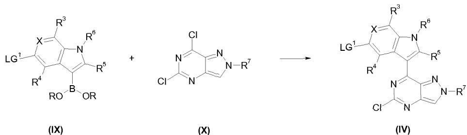
5 Scheme 4 illustrates a method of preparing intermediates of Formula (IV), wherein R<sup>3</sup>-R<sup>7</sup> and X are as defined in Formula (I) and LG<sup>1</sup> is as defined above. Heating intermediates of Formula (X) with boronates of Formula (IX) under palladium-catalyzed Suzuki coupling conditions, using for example Pd(PPh<sub>3</sub>)<sub>4</sub>, Na<sub>2</sub>CO<sub>3</sub> in water and 1,4-dioxane as solvent, yields intermediates of Formula (IV).
