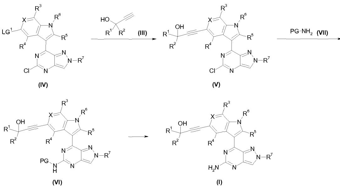
Scheme 2 illustrates a further method of preparing compounds of Formula (I), wherein R<sup>1</sup>-R<sup>7</sup> and X are as defined in Formula (I). Intermediates of Formula (IV) can be reacted with alkynes of Formula (III) under palladium-catalysed Sonogashira coupling conditions, using for example Pd(PPh<sub>3</sub>)<sub>4</sub>, CuI and a base such as Et<sub>3</sub>N in acetonitrile,
