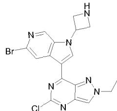
A stirred solution of intermediate 34 (1.79 g, 3.36 mmol) in DCM (20 ml) under a nitrogen atmosphere at ambient temperature was treated with TFA (2.0 ml, 26.1 mmol), and the resulting mixture was stirred for 1 hour. The mixture was concentrated *in vacuo* to afford the desired product (1.84 g, 100%).
