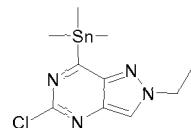
20 A degassed mixture of 5,7-dichloro-2-ethyl-2H-pyrazolo[4,3-d]pyrimidine (0.10 g, 0.46 mmol), hexamethylditin (0.30 g, 0.92 mmol), tetrakis(triphenylphosphine)palladium(0) (0.03 g, 0.023 mmol) and 1,4-dioxane (6.0 ml) under an argon atmosphere was heated at 80 °C for 7 hours. The mixture was cooled to ambient temperature, filtered through Celite® and the filtrate concentrated *in vacuo* to afford the desired product as a brown solid (0.17 g, 100%).
