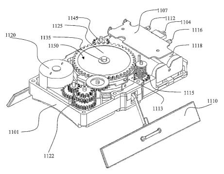
(57) Abstract: The present invention provides a device for enhancing circulation by intermittently tightening and relaxing a closure encircling a limb. The device comprises a continuously operating motor, at least one rotating element and a mechanism driven by the motor for intermittently rotating the rotating element in a first direction to tighten said closure and in a second opposite direction to relax said closure, thereby applying a cyclic pressure on the limb.
