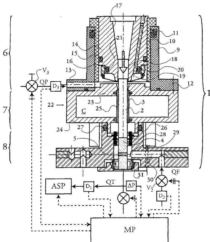
(57) Abstract: The invention concerns a sample-holder (1) for measuring parameters of porous objects, comprising a draft cell including a microwave frequency (C), through which the object passes so as to be able to measure moisture content before and/or after measuring draft.
