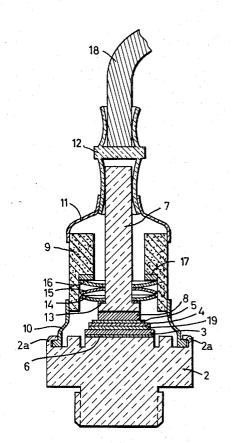
3,378,735 SEMICONDUCTOR DEVICE HOUSING WITH SPRING CONTACT MEANS AND IMPROVED THERMAL CHARACTERISTICS
