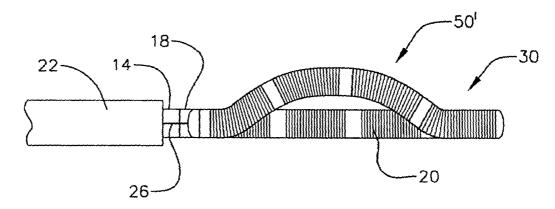
(57) Abstract: A probe that includes a elongate body (12) and a steerable loop structure (30, 74) that supports electrodes (20) or other operative elements against the body tissue.
