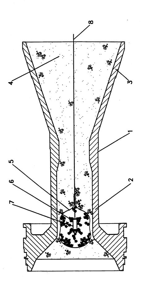
FOAMED IN PLACE IGNITER AND AFT-END ASSEMBLY FOR ROCKET MOTOR COMPRISING THE SAME
