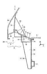
a raising part connecting the cup and only a portion of the side member, having a width, measured in a longitudinal direction of the vehicle, substantially equal to that of the cup.
