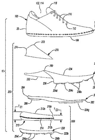
outer sole member also includes a rib extending downwardly from the upper portion and defining a cavity.
